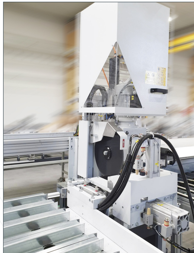
Saw with Servofeed and Vario-Material clamping
