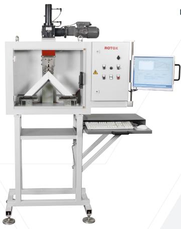
The corner testing device is one of the important quality testing devices in the window production.
