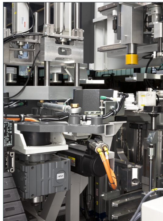
Optional: Motor-driven swivelling device, NC controlled support shifting
