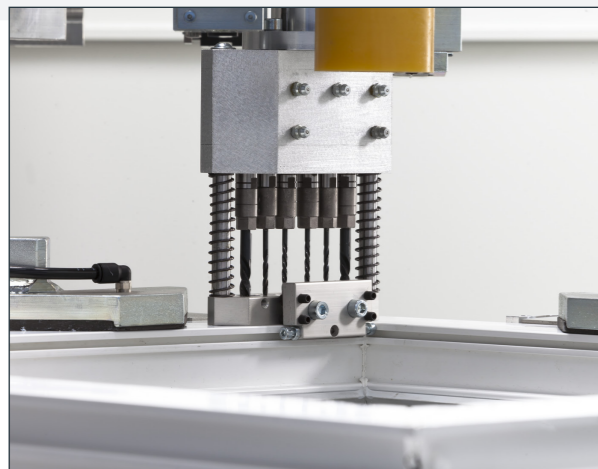
Swivelling corner and rebate stay hinge unit with electric motor for a maximum drilling performance
