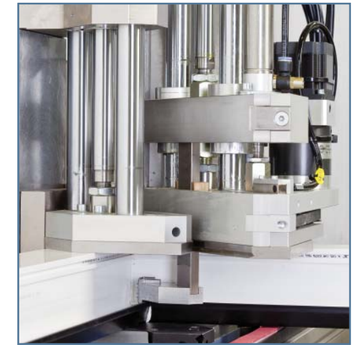
Motor moveable sealing forming units pushing and pulling
